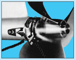
■ Cuts line with each revolution (forward or reverse), with no loss of speed and efficiency
